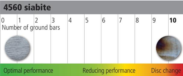
\* Tested on stainless steel bars Ø 20mm, # 60, 10 sec. on each bar. Manual test. Turbo Backing Pad II. 1100W angle grinder.
